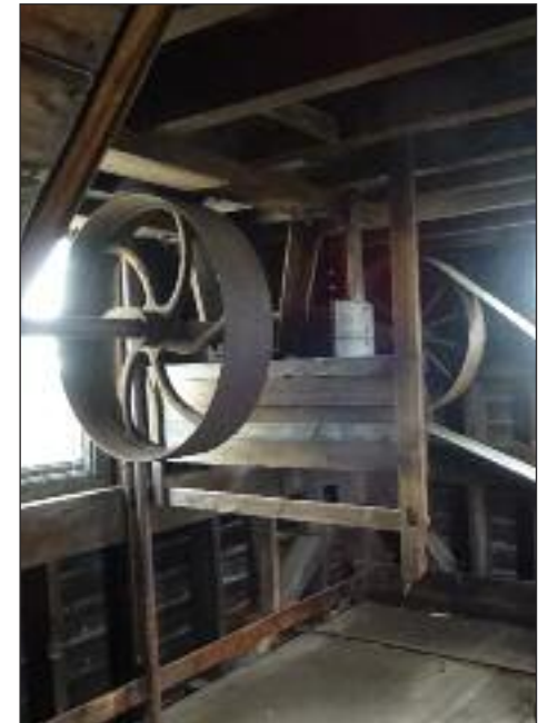
Victorian hoist equipment installed in the Jubilee tower in 1897 to move grain around the site
